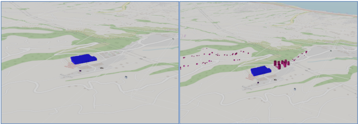
Figure 33. A tile and its child rendered using additive method
