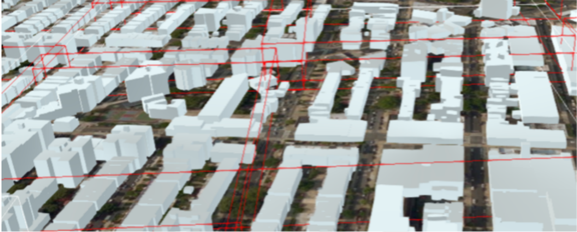
Figure 20. Tile borders overlap and features are always completely inside of a node.
